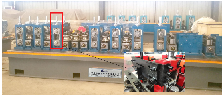
FIGURE-3 , The bracket is installed on the first fin pass
